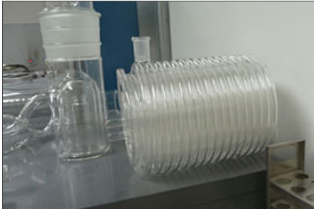
This piece, which coils 75 feet of tubing into a package the size of a coffee can, took six weeks to shape.
