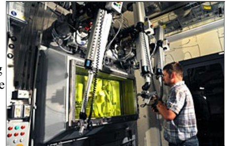
The irradiation assisted stress corrosion cracking (IASCC) test rig at INL's Materials & Fuels Complex.
